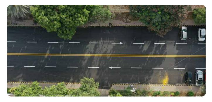
In Karachi, where Shell House is located Shell Pakistan constructed a plastic infused road surface. The road is 730 feet long and 60 feet wide and the surface contains recycled material from discarded Shell lubricant bottles. This is a purpose-built solution which is a benefit for Shell, neighboring residents, schools and the church community.
